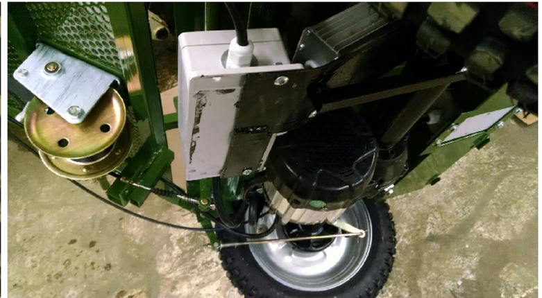
Control Box and Skid Plate After Bending
